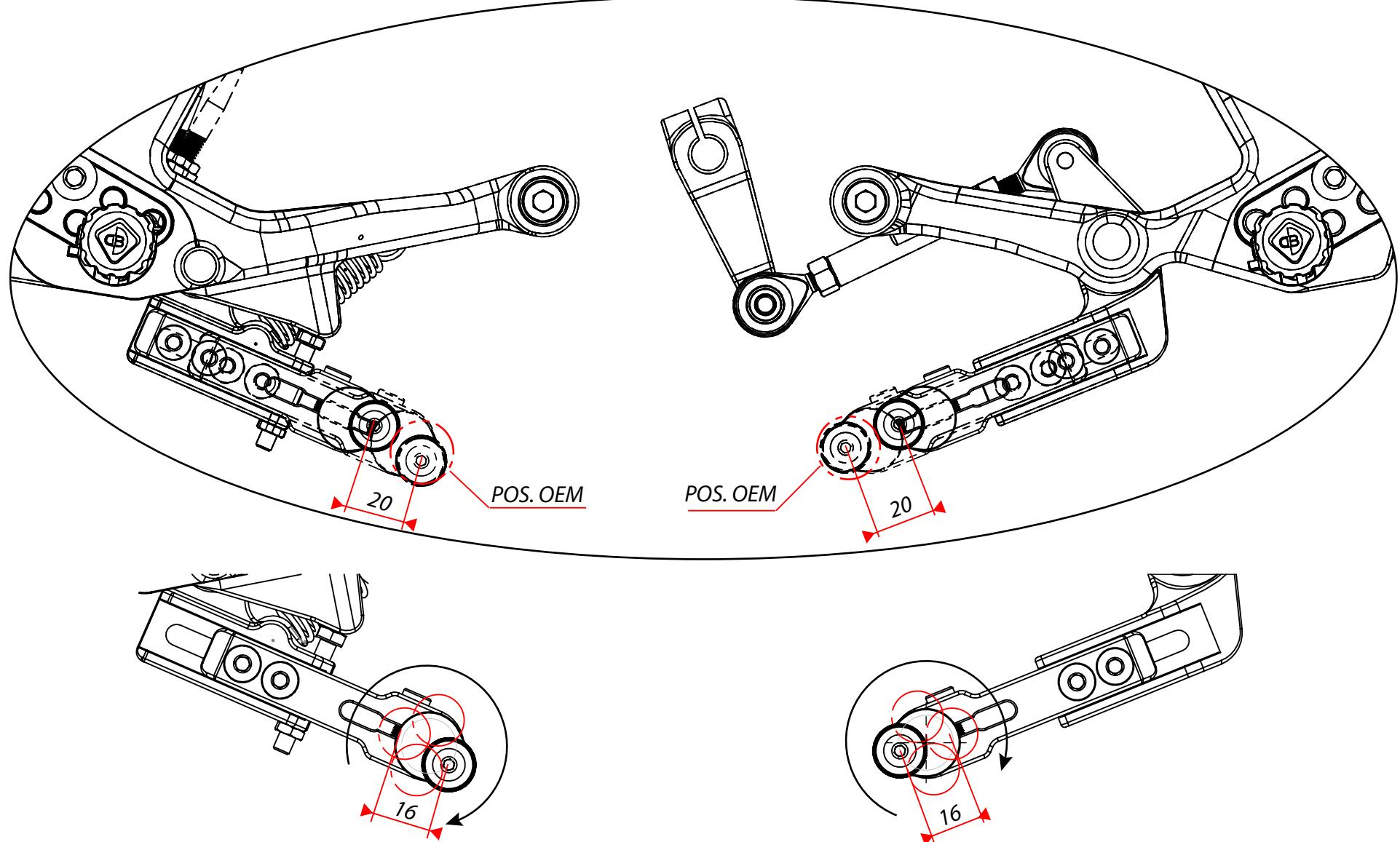
RAPPRESENTAZIONE MONTAGGIO CAMBIO NORMALE / **STANDARD SHIFT ASSEMBLY ILLUSTRATION**
