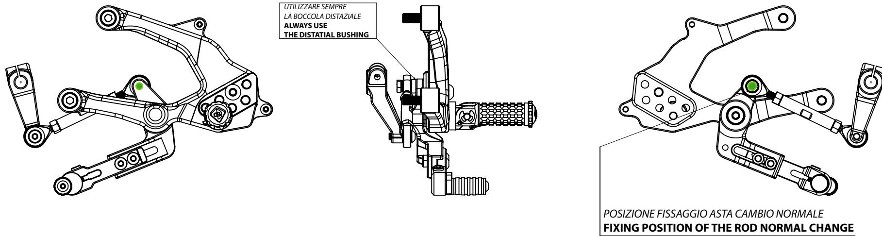
RAPPRESENTAZIONE MONTAGGIO CAMBIO ROVESCIO / **REVERSE SHIFT ASSEMBLY ILLUSTRATION**
