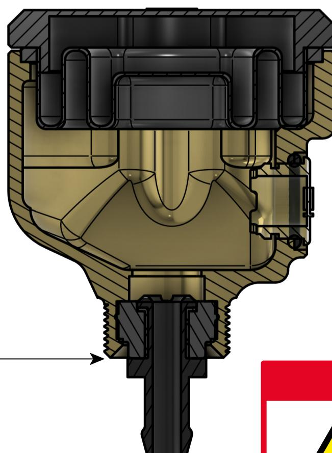
2) Make sure that the edge of the plastic fitting is fully exposed outside the rubber.
