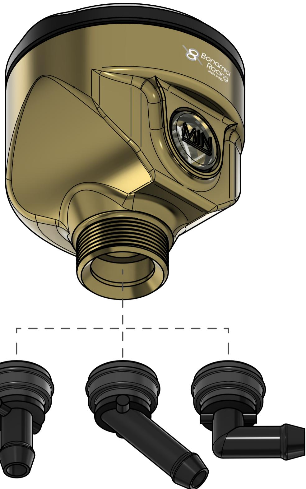
3) Insert the plastic fitting up to the indicated position without removing the rubber and without using any tools that could cause damage. Use DOT 4 oil as a lubricant. After assembly, wash and rinse thoroughly.
